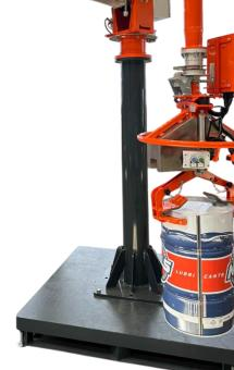
The customized configuration of the ATISmirus 300 manipulator with pneumatic clamp system was specifically designed to meet the needs of drum handling. The flexibility of the gripper, combined with the manipulator's capacity, allows for safe and efficient process management.
